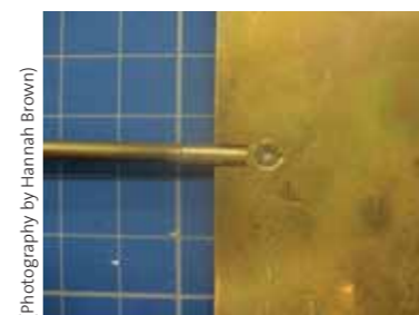
Figure 2. Attaching the removable arm in place to the back plate with an M2 screw
