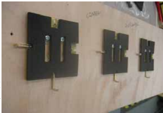
Figure 5. Checking the location of the screws in the 'keyholes' cut into the back plate
