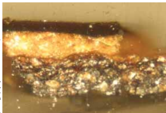
Figure 3c. Cross-section (as in figure 3a) after staining with Lugol's solution, VIS light. Adhesion failure at the interface between the top foundation and the starch-containing layer
