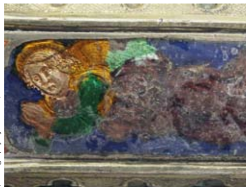
Figure 2. (M.580-1910) Detail of the coating as it lifts from a basse taille enamel plaque
