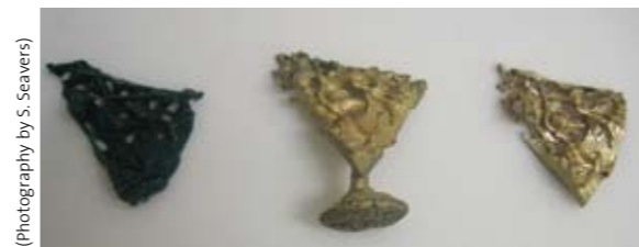
Figure 4. (From left) Wax cast, unfinished casting (centre), finished casting (right)
